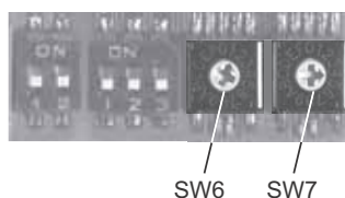
Fig. 8 Setting the BACnet MAC address
