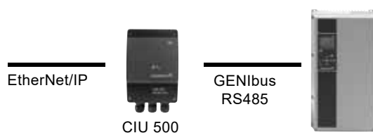
Fig. 2 Example of a CIU 500 solution. The figure shows a CUE drive for pumps.
