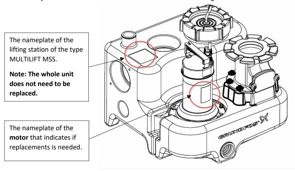
2. Check the nameplate of the lifting station unit:
