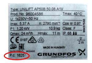
The first two numbers indicate the production year (16 for 2016) and the last two numbers indicate the production week (week 25) in this example.
