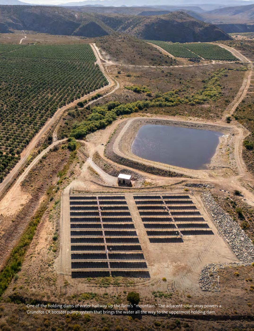
One of the holding dams of water halfway up the farm's "mountain." The adjacent solar array powers a Grundfos CR booster pump system that brings the water all the way to the uppermost holding dam.
