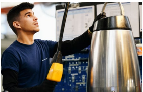
Front page photo: A Grundfos colleague operates a crane to lift an SE pump. SE pumps are designed for handling wastewater, process water and unscreened raw sewage in heavy-duty municipal, utility and industrial applications.
